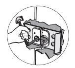
Use Kason No. 1145 hexagonal wrench for easy locking of all Kason panel fasteners.
