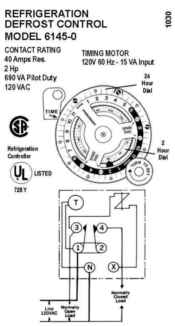
To Set: Screw pins into dial at time defrost is desired. (Four hours minimum time between pins.)
