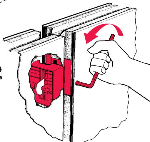
4. After curing, panels are read for assembly. Completed panels are easily locked in position at assembly site using the Kason No. 1145 wrench.
