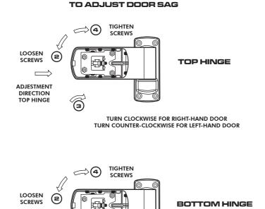
TURN COUNTER-CLOCKWISE FOR RIGHT-HAND DOOR TURN CLOCKWISE FOR LEFT-HAND DOOR
